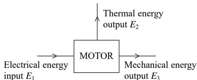
The efficiency of the motor is
