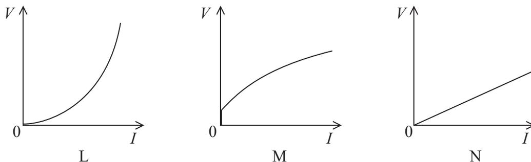
The three components are a metal wire at constant temperature, a filament lamp and a diode.
